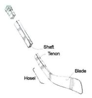
Note: Because most foam sealants are flammable, filling the Gopher blade's "external" tenon with foam sealant and then jamming the shaft into it was NOT tried, due to the necessity of also heating the external tenon to fit the shaft. I was using an open flame and didn't want to, oh say, *ignite* everything.
